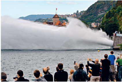
Photo: Yves Favre, Keystone, August 2009. Every 10-12 years, the Company tests its sluice gates. During the 2009 exercise, 6 million litres of water were poured into Lake Geneva in 5 minutes. With a flow of 20 000 litres per second, the transient jet of water achieved a length of 300 metres.
